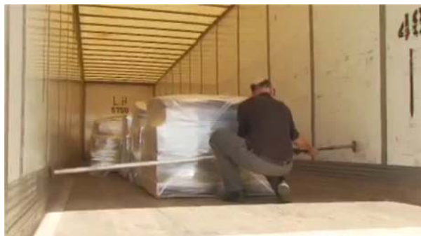
Figure 5. Securing pallets to prevent shifting of the load during transport
