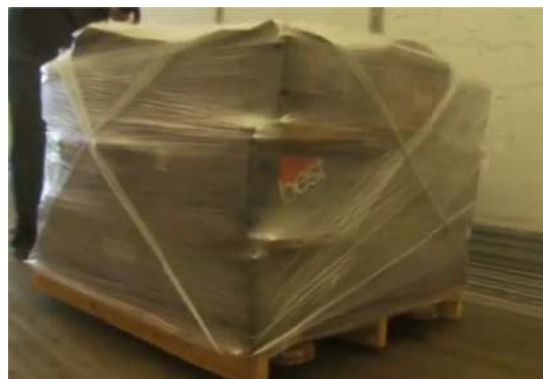
Figure 4. Batteries secured to the pallet with stretch wrap
