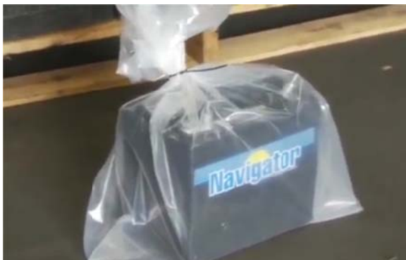
Figure 3. Damaged batteries that are not visibly leaking electrolyte must be put in heavyweight polyethylene plastic bags
