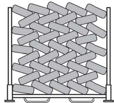
Figure 1. Typical laced storage<sup>(3,4)</sup>
